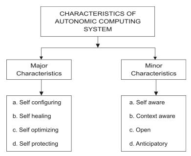
Fig. 1: Characteristics of Autonomic Computing System
