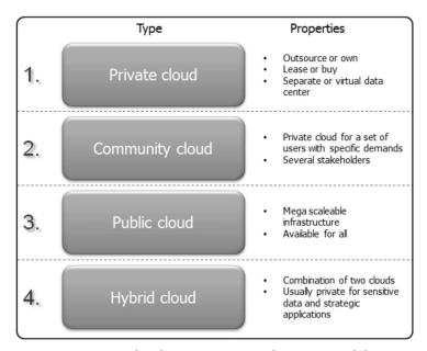
Figure 1: Cloud Computing Deployment Model
